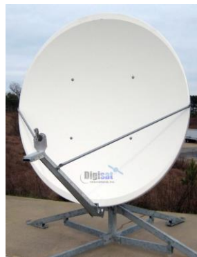
Fig.2. VSAT Outdoor unit
